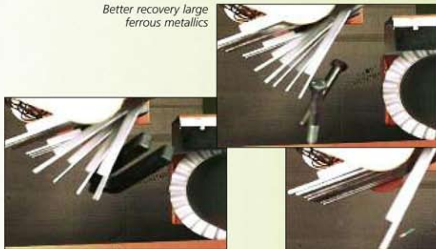
Powerful inverted paddles deflect heavy (8 lbs) metal objects into sorting stations
